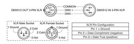
**Special Note: Line Termination.** When longer runs of cable are used, you may need to use a terminator on the last unit to avoid erratic behavior. A terminator is a 110-120 ohm 1/4 watt resistor which is connected between pins 2 and 3 of a male XLR connector (DATA + and DATA -). This unit is inserted in the female XLR connector of the last unit in your daisy chain to terminate the line. Using a cable terminator (ADJ part number Z-DMX/T) will decrease the chances of erratic behavior.
